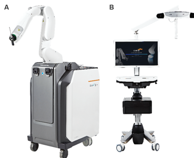
Fig. 1 Composition of CUVIS-joint active robotic system. (A) Robotic arm. (B) Main console.
